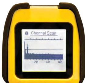
Radio signal strength indication to map radio conditions in the operating zone
